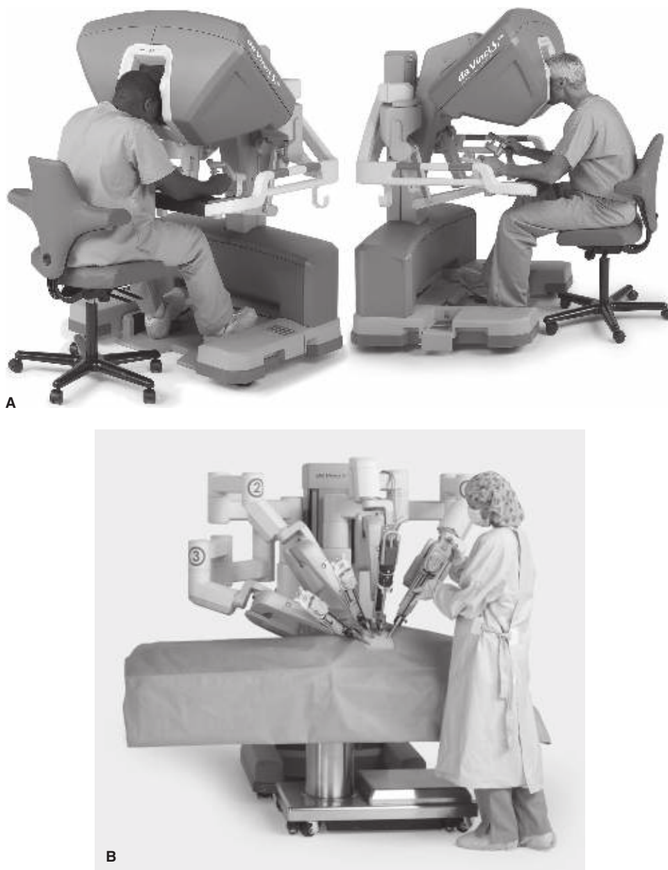
▲ Figure 11-1. The da Vinci Si robotic surgical system made by Intuitive Surgical Inc. It consists of the (A) surgeon console (here with the dual console HD Si) and (B) patient-side surgical cart, in this model with four arms. (Used with permission from Intuitive Surgical Inc.).
